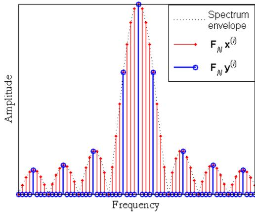
Fig. 3. Spectral illustration of IFDMA ( $N=64$ ,  $K=4$ ).
