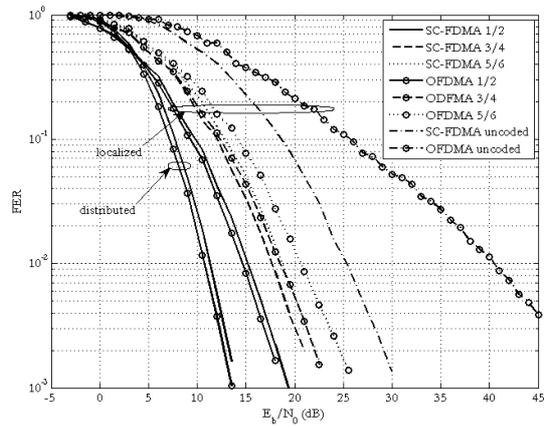
Fig. 4. SC-FDMA vs. OFDMA performance with QPSK and 5 RBs.
