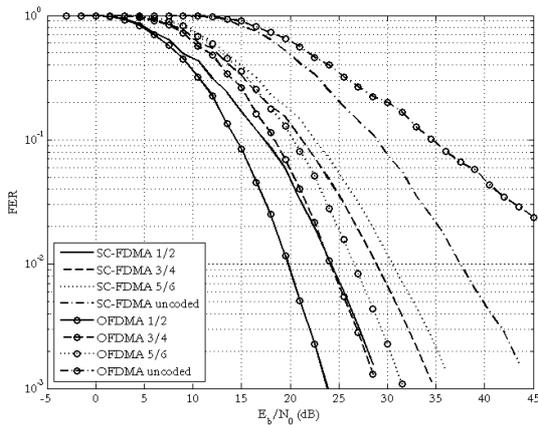
Fig. 6. SC-FDMA vs. OFDMA, 64-QAM, 5 localized RBs.
