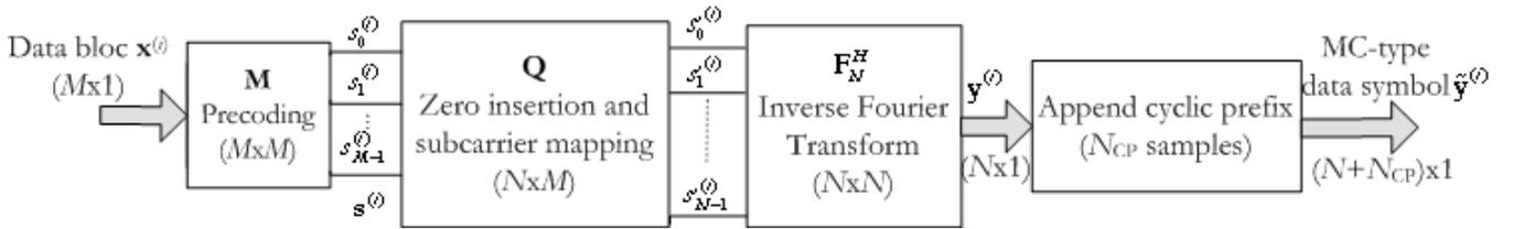
Fig. 1. Generalized MC transmitter for SISO transmission.
