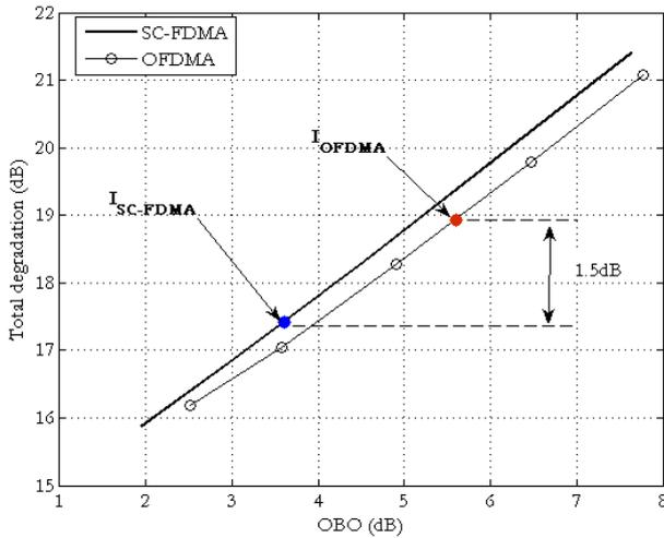
Fig. 8. Total system degradation of OFDMA and SC-FDMA, QPSK 1/2, 5 localized RBs, target FER 1%, Rapp HPA.
