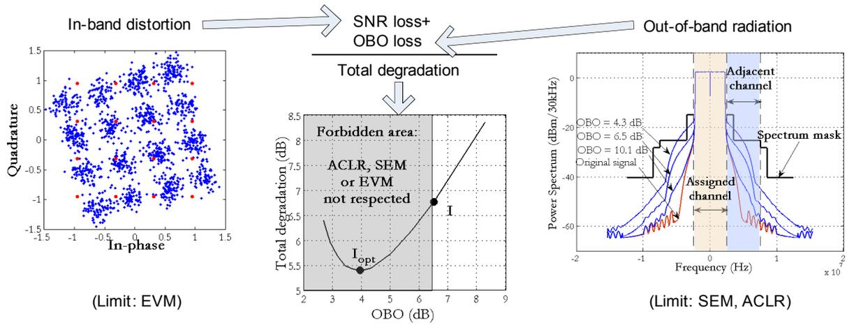
Fig. 7. Illustration of nonlinear distortion in an uncoded OFDMA system with 16-QAM signal mapping.
