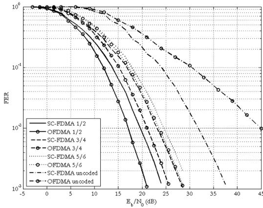
Fig. 5. SC-FDMA vs. OFDMA, 16-QAM and 5 localized RBs.
