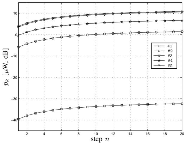
Fig. 8. Transmit power as a function of the iteration step.
