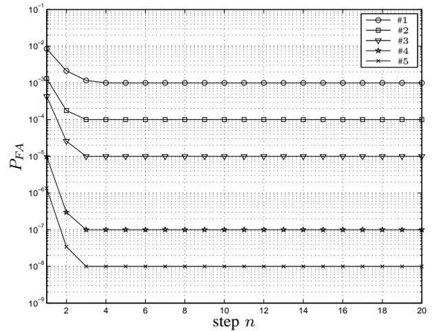
Fig. 10. Probability of false alarm as a function of the iteration step.
