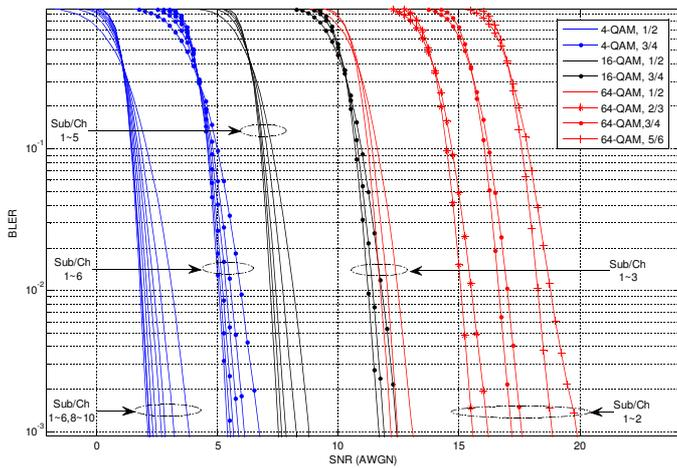
Fig. 2. Simulated performance on AWGN for the 32 WiMax compatible CTC Tx-modes.
