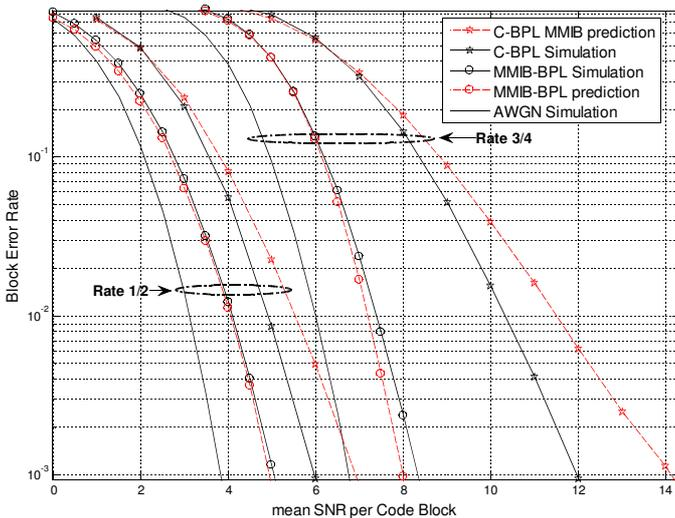
Fig. 3. Simulated BLER performance and prediction for two CTC modes with and without bit&power loading.
