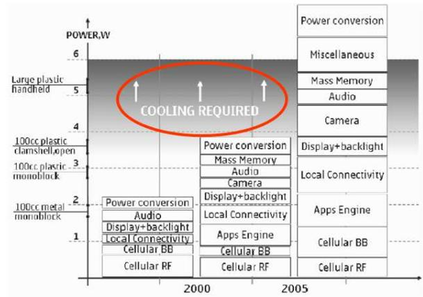
Fig. 6. Power consumption increase in wireless terminals<sup>6</sup>
