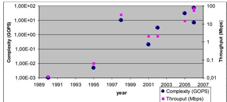
Fig. 5. Throughput and complexity trends for wireless standards
