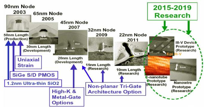
Fig. 1. Technology nodes and predicted end of CMOS down-scaling with possible alternatives (nanotubes and nanowires) for post-2015 nanotechnology<sup>2</sup>
