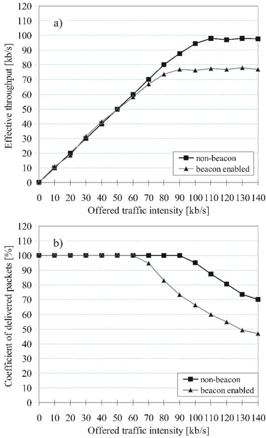
Fig. 2. Bidirectional transmission in a system consisting of two nodes: a) intensity of the operated traffic, b) coefficient of delivered packets
