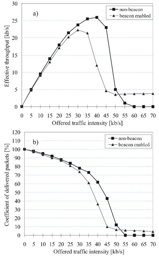
Fig. 4. Unidirectional transmission in a system containing hidden stations: a) intensity of the operated traffic, b) coefficient of delivered packets
