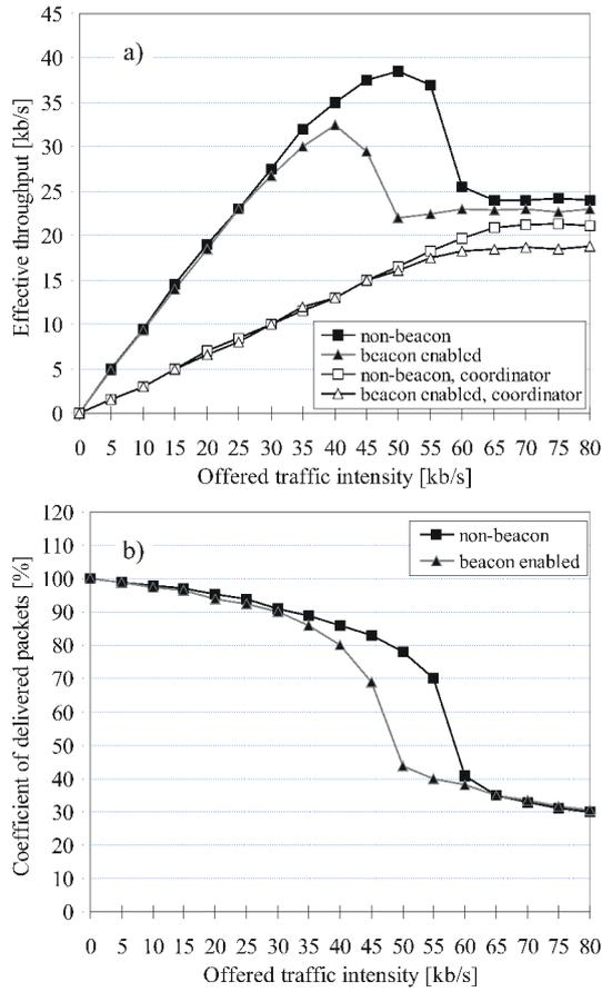
Fig. 5. Bidirectional transmission in a system containing hidden stations: a) intensity of the operated traffic, b) coefficient of delivered packets
