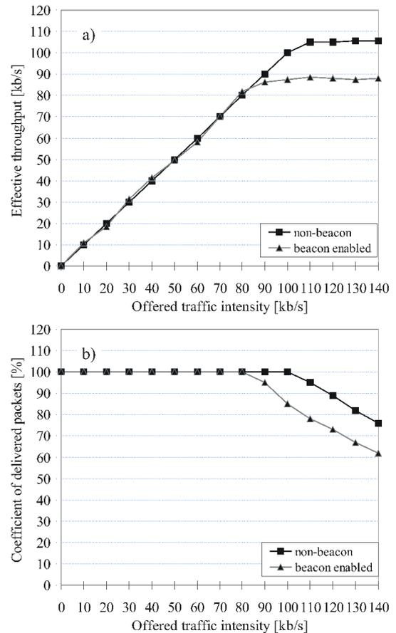
Fig. 1. Unidirectional transmission in a system consisting of two nodes: a) intensity of the operated traffic, b) coefficient of delivered packets
