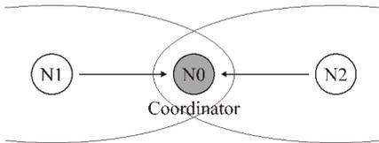
Fig. 3. Model of a system containing hidden stations
