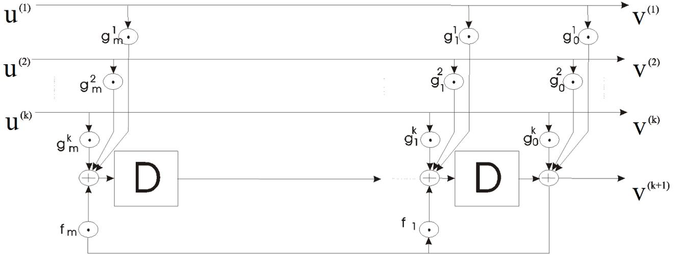
Fig. 1. Systematic feedback convolutional encoder over ring of integers modulo-M.
