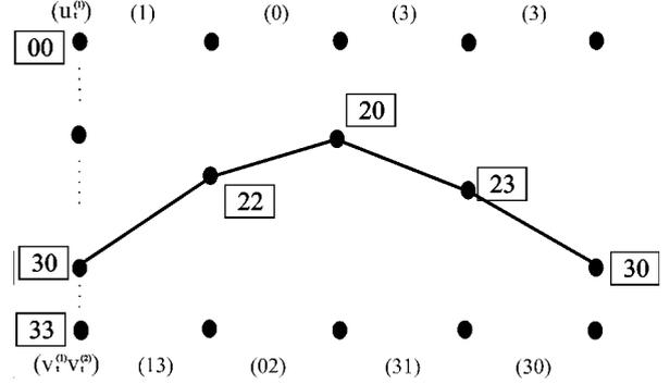
Fig. 4. Tree diagram for proper encoding process for tailbiting codes over ring  $Z_4$ .
