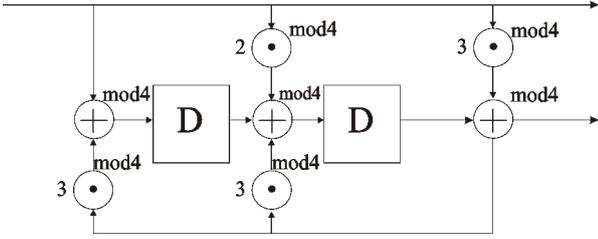
Fig. 2. Encoder of the convolutional code  $G(D) = \begin{bmatrix} 1 & \frac{3+2D+D^2}{1+3D+3D^2} \end{bmatrix}$  from the example.
