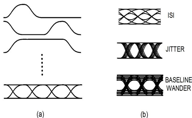
Fig. 1. The idea of the eye diagram construction (a), and common eye distortions (b).
