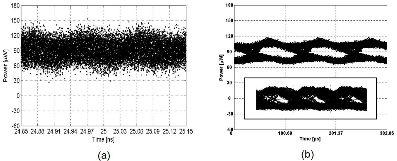
Fig. 5. Eye diagram of weak signal register directly on the oscilloscope (a), and using the described system (b).
