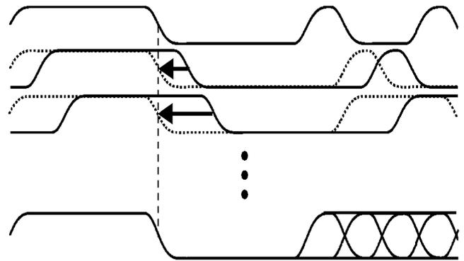
Fig. 4. Aligning of patterns shifted by transmission delay variation.
