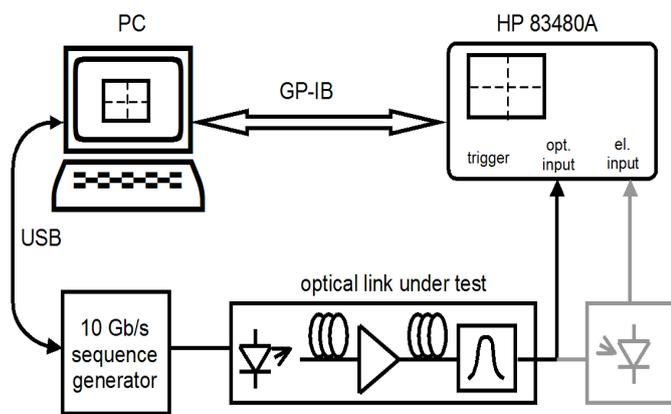
Fig. 3. Block diagram of measurement system.
