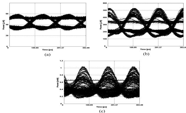
Fig. 6. Eye diagram obtained at the end of same optical link for varying EDFA amplification.
