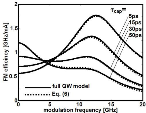
Fig. 3. Comparison of FM efficiency obtained from full QW model and from (6).
