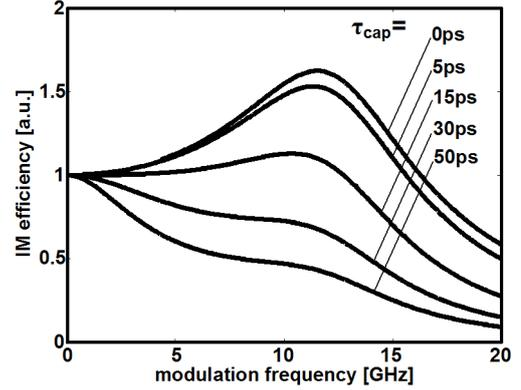
Fig. 1. IM efficiency  $|\delta P / \delta I|$  versus modulation frequency and capture time.
