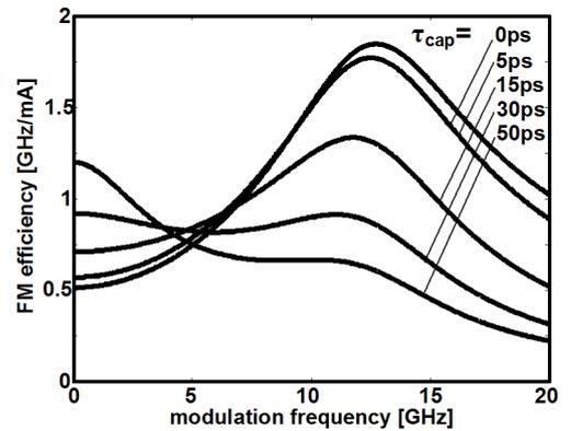
Fig. 2. FM efficiency  $|\delta \nu / \delta I|$  versus modulation frequency and capture time.
