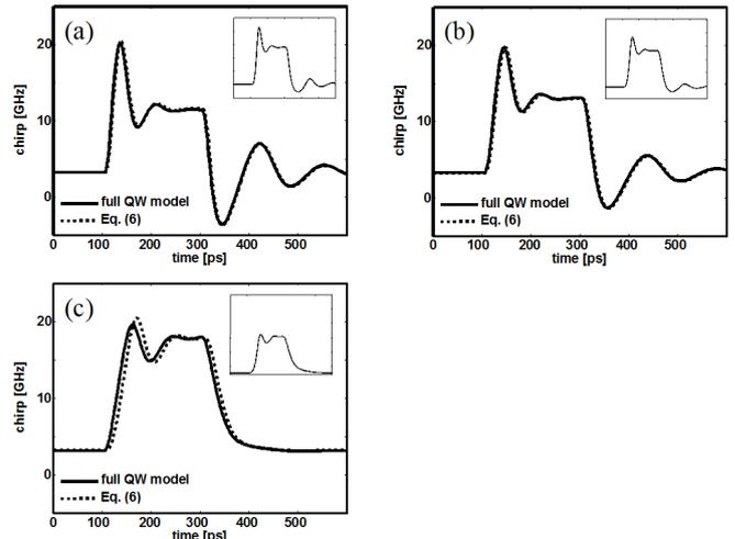
Fig. 4. Comparison of time domain chirp evolution obtained from full QW model and from (6); capture time equal to 5 ps (a), 15 ps (b) and 50 ps (c). In the insets corresponding power waveforms.
