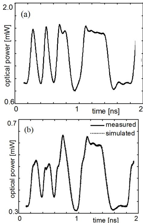
Fig. 5. Modulated laser output power (a), and fiber output power corrupted by interplay of the laser chirp and the fiber chromatic dispersion (b).
