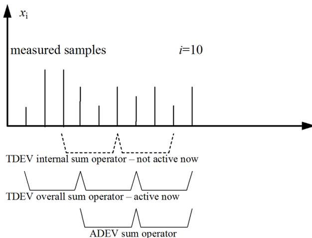
Fig. 4. Joint real-time ADEV and TDEV calculation for observation interval  $3\tau_0$ , sample number 10 is measured.
