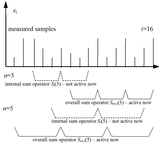
Fig. 2. Real-time TDEV calculation for observation intervals observation intervals  $3\tau_0$  and  $5\tau_0$ , sample number 16 is measured.
