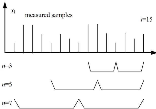
Fig. 1. Real-time ADEV calculation for observation intervals observation intervals  $3\tau_0$ ,  $5\tau_0$ ,  $7\tau_0$  sample number 15 is measured.
