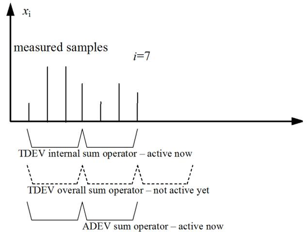
Fig. 3. Joint real-time ADEV and TDEV calculation for observation interval  $3\tau_0$ , sample number 7 is measured.
