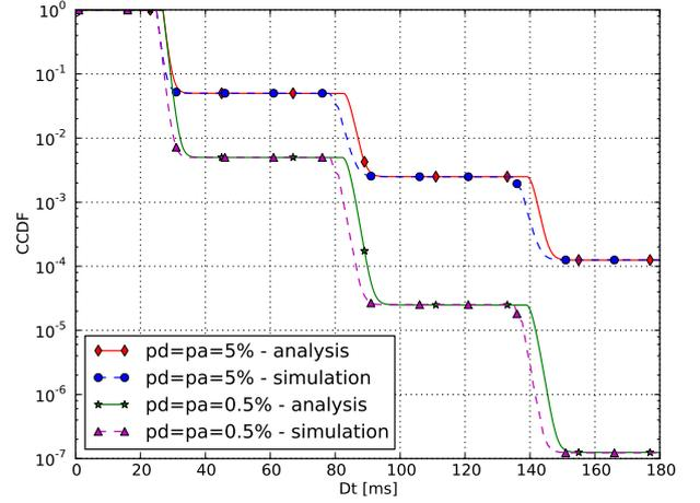
Fig. 6. Complementary CDF of time  $Dt$  for case#1: VC with low packet transfer delay variation.
