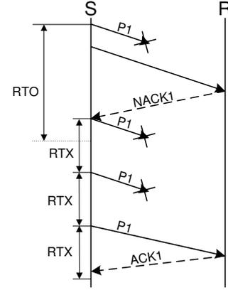
Fig. 5. The Virtual Link retransmission schema.
