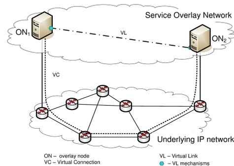
Fig. 1. The Virtual Link concept.
