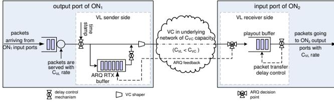
Fig. 2. The mechanisms of Virtual Link.
