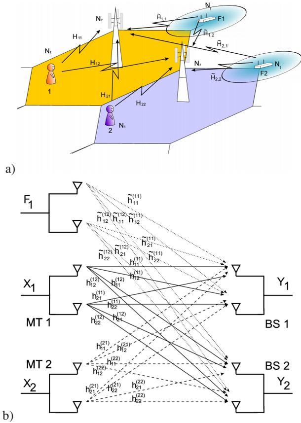
Fig. 1. MIMO interference channel: general 2-cell 2-user model with interfering femtocell AP
