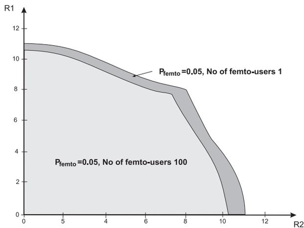
Fig. 6. Achieved rate region for TSD-MIMO for  $P_{femto} = 0.05$ ; number of femtocells equals 1 (case A) and 100 (case B)
