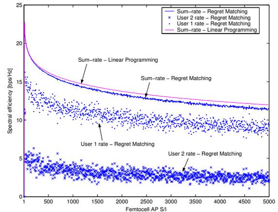
Fig. 4. Achieved rates vs. femtocell AP power to noise ratio in case of SVD-MIMO
