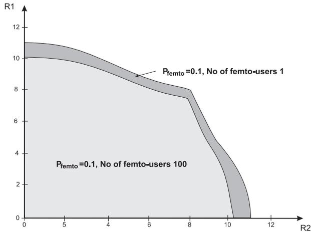
Fig. 5. Achieved rate region for TSD-MIMO for  $P_{femto} = 0.1$ ; number of femtocells equals 1 (case A) and 100 (case B)
