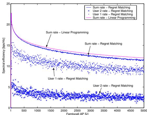
Fig. 3. Achieved rates vs. femtocell AP power to noise ratio in case of TSD-MIMO
