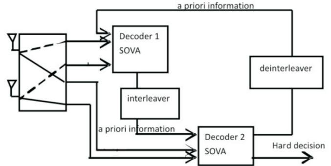
Fig. 4. Space-Time Turbo Decoder
