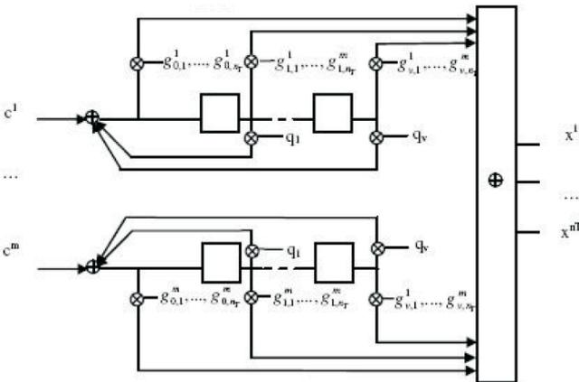
Fig. 3. Block diagram of a recursive STTC encoder for M-ary modulation
