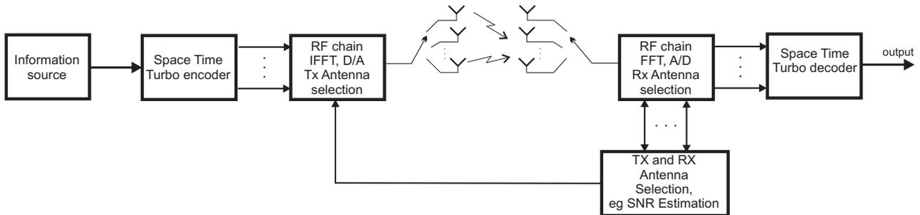
Fig. 1. Block diagram of the MIMO-OFDM system with transmit and receive antenna selection and optionally with space time coding
