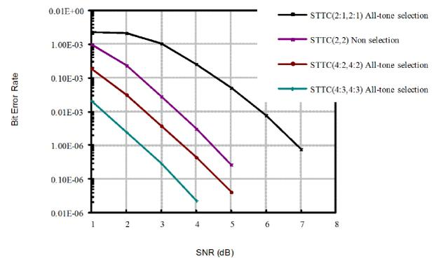
Fig. 5. STTC-OFDM system with all-tone transmit/receive antenna selection
