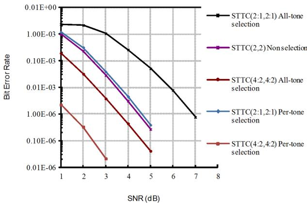
Fig. 6. Comparison of all-tone and per-tone selection methods in STTC-OFDM system
