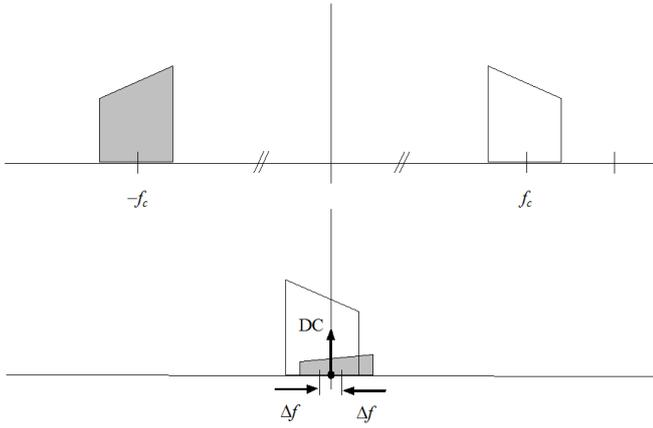
Fig. 2. Power spectrum for a direct-conversion receiver.
