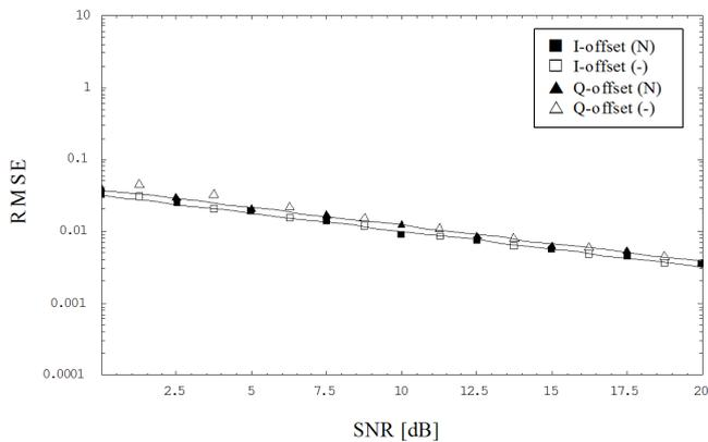
Fig. 5. Root-mean-square error of DC offset estimates:  $L = 500$ ,  $g_R = 1.2$ ,  $\varphi_R = 10^\circ$ ,  $\theta_0 = 45^\circ$ ,  $v_0 = 0.1$ ,  $d_I = d_Q = 0.1$ .
