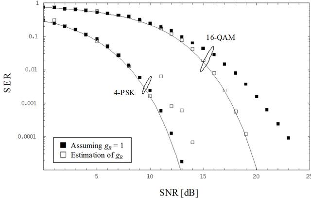
Fig. 7. Evolution of the symbol error rate (evaluation of noise power skipped):  $L = 500$ ,  $g_R = 1.2$ ,  $\varphi_R = 10^\circ$ ,  $d_I = d_Q = 0.1$ .
