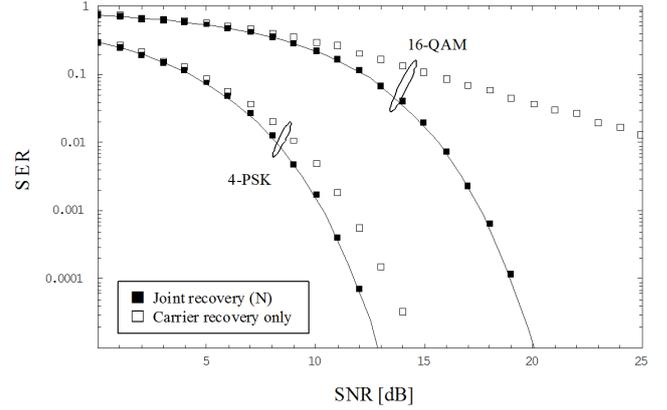
Fig. 6. Evolution of the symbol error rate (noise power assumed to be known):  $L = 500$ ,  $g_R = 1.2$ ,  $\varphi_R = 10^\circ$ ,  $d_I = d_Q = 0.1$ .
