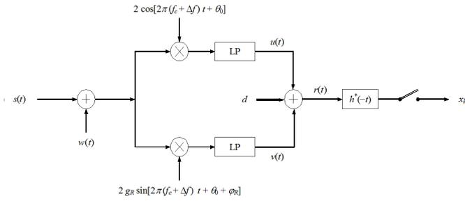
Fig. 1. Basic block diagram of the IQ demodulator architecture.
