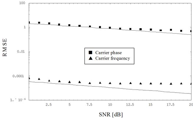
Fig. 3. Root-mean-square error of carrier frequency and phase estimates:  $L = 500$ ,  $g_R = 1.2$ ,  $\varphi_R = 10^\circ$ ,  $\theta_0 = 45^\circ$ ,  $v_0 = 0.1$ ,  $d_I = d_Q = 0.1$ .
