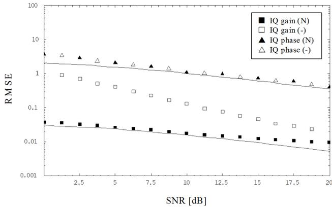
Fig. 4. Root-mean-square error of IQ gain and phase estimates:  $L = 500$ ,  $g_R = 1.2$ ,  $\varphi_R = 10^\circ$ ,  $\theta_0 = 45^\circ$ ,  $v_0 = 0.1$ ,  $d_I = d_Q = 0.1$ .
