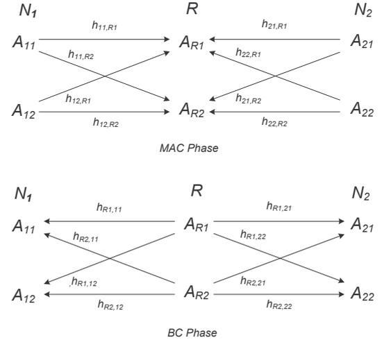
Fig. 1. Two-way relaying scheme employing Alamouti's STBC at each node.
