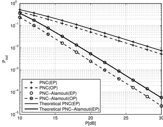
Fig. 2. Outage probabilities for uncoded and Alamouti coded TWR using PNC protocol (EP: Equal power, OP: Optimal Power)
