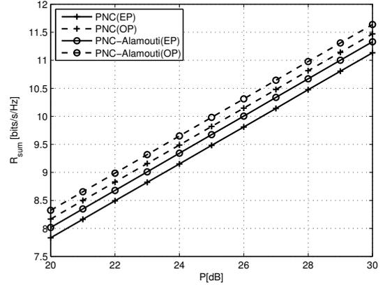
Fig. 3. Sum-rates for uncoded and Alamouti coded TWR using PNC protocol (EP: Equal Power, OP: Optimal Power).
