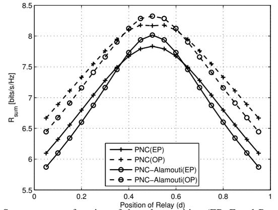
Fig. 4. Sum-rates as a function of the relay position (EP: Equal Power, OP: Optimal Power).
